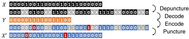
Figure 23: An example of the BCC decoding and regeneration at 3/4 coding rate.
