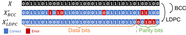
Figure 8: Distribution of coding errors (mismatch between X and X' ), for BCC and LDPC, respectively.
